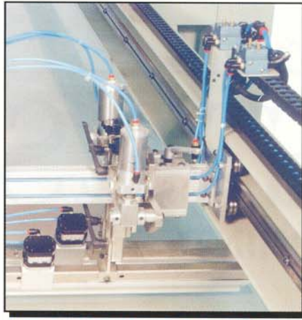
Heavy duty squeegeelizer cylinders and adjusting position control
