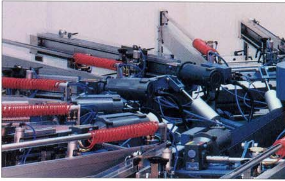
Electro-mechanical drive systems provide smooth print/flood strokes despite image size.
