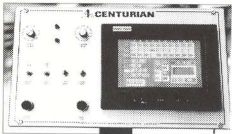
State-of-the-Art PLC Controller features on-line production and troubleshooting data.
